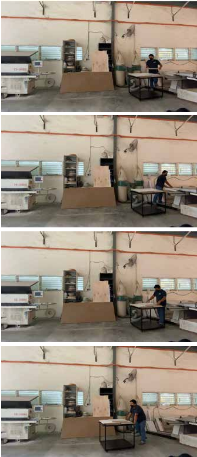
Figure 3: Lifting activity conducted using proposed industrial ergonomic trolley-lifter by the worker
