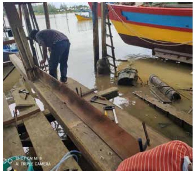
Figure 7: A Boatbuilder Attaching the Planks onto the Keel
