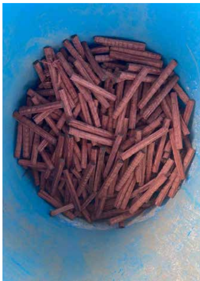
Figure 3: Trunnels Used to Strengthen Boat Walls
