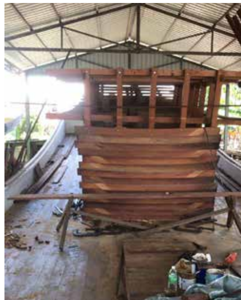
Figure 20: The Construction of the Cabin
