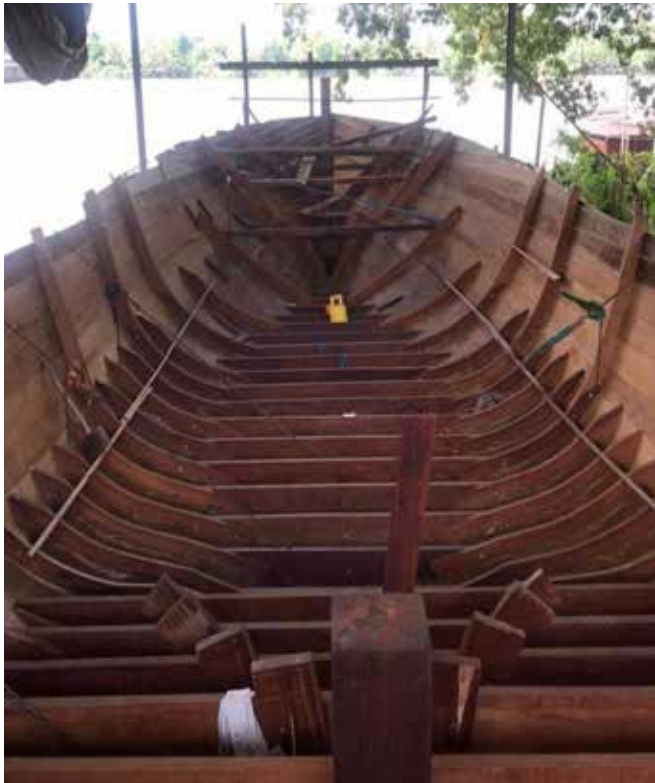
Figure 14: Planks have been Attached to Form the Boat Wall
