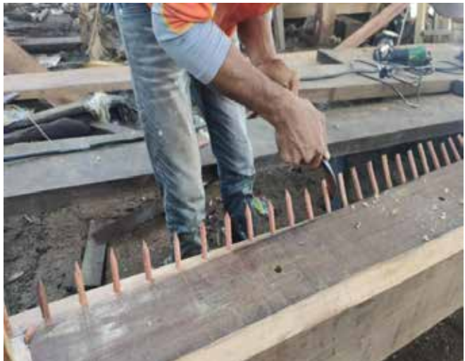
Figure 9: Sickles are Used to Produce Pointed Trunnels
