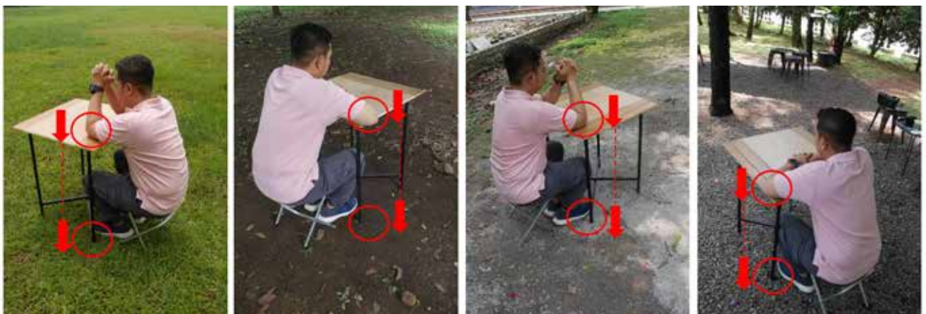
Figure 9. Condition of each table when in use and when under load on (1) grass, (2) ground, (3) sand, (4) gravel
