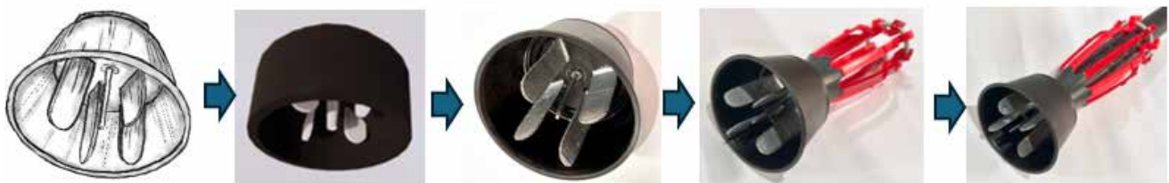
Figure 18. Table Stabilizer Design on The Sand Surface design step outcomes
